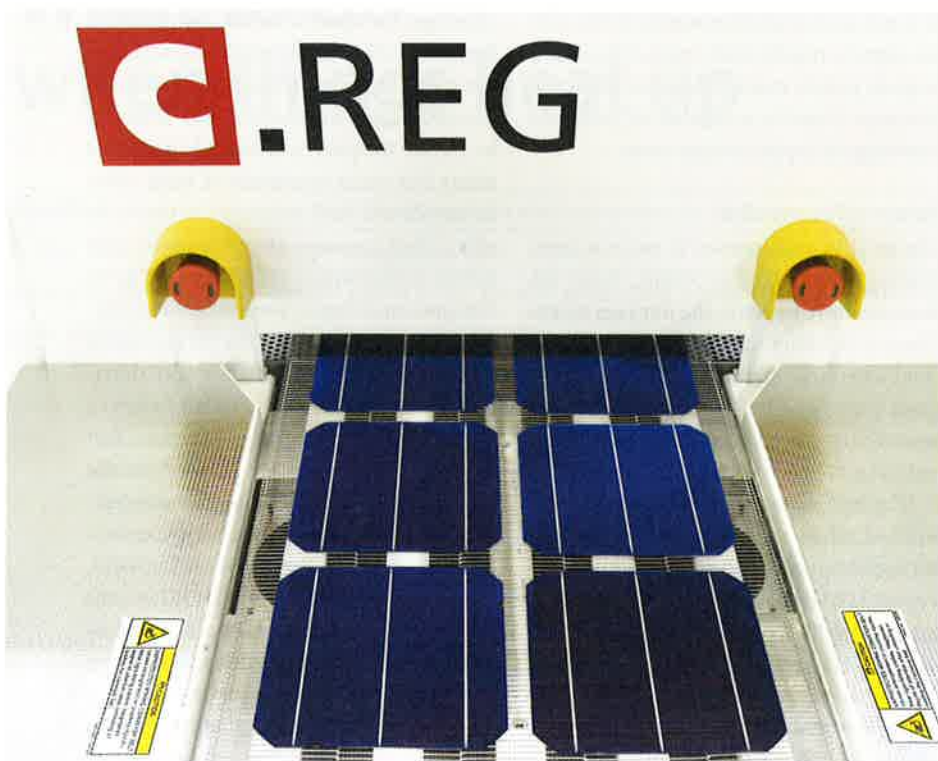
Centrotherm's C. Regeneration tool is a modified belt furnace with the ability to condition monocrystalline cells in order to reduce instances of LID – light-induced degradation.
